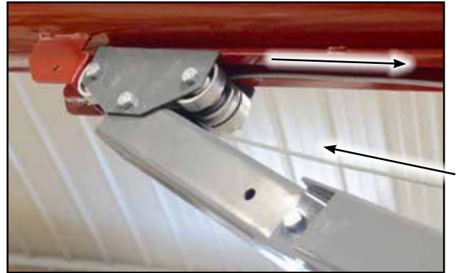
Fig 33 - Cable around trolley roller
