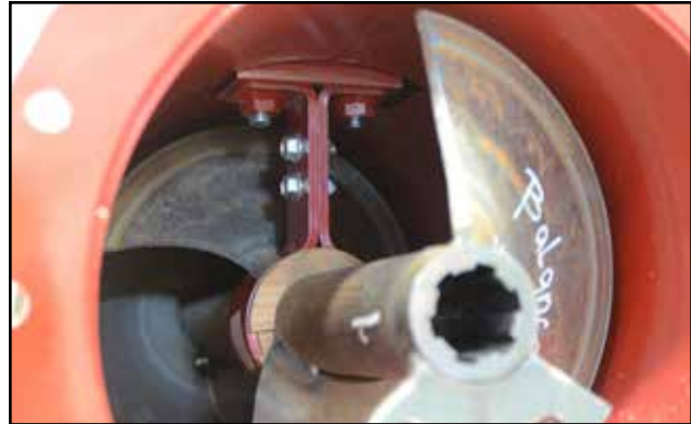
Fig 27 - Hanger bearing from end of tube
