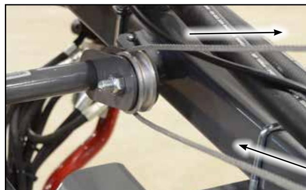
Fig 32 - Cable roller on main frame
