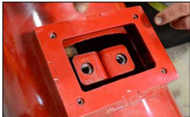
Fig 44 - Hanger bearing without covers
