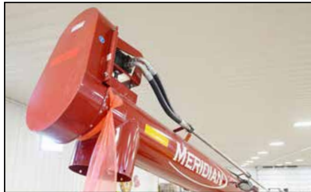
Fig 12 - Hydraulic drive for auger flighting
