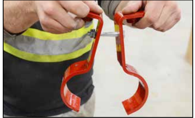
Fig 45 - 2 inch bolt joining the brackets
