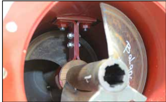
Fig 42 - Hanger bearing installed inside tube
