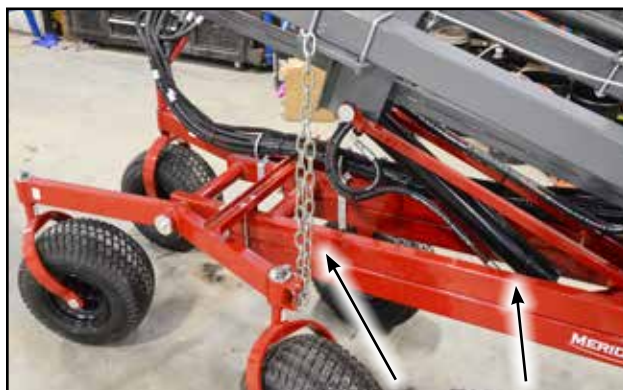
Fig 17 - Walking Beam transport chain and lift cylinder
