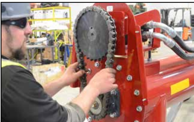
Fig 36 - Inspect chain and sprockets
