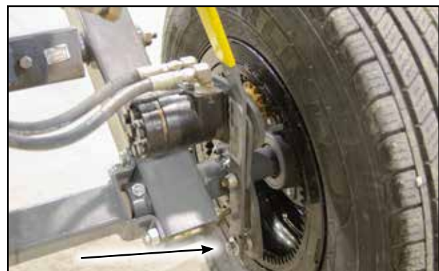
Fig 38 - Flange nut at bottom of assembly
