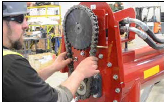
Fig 29 - Inspect chain and sprockets
