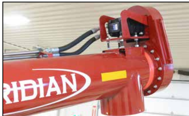
Fig 13 - Discharge-end hydraulic drive
